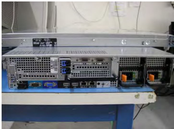
Figure 2. VOD 125/300W (Dell 2950 – Rear View)
