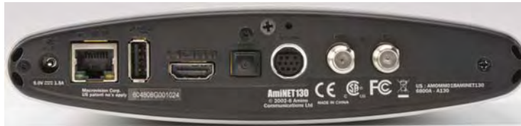
Figure 2. AmiNET130 Rear Panel (left to right)
