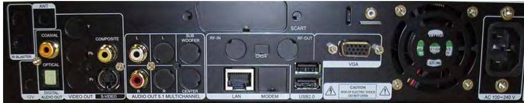
Figure 2. WM IPR – Rear Panel Connectors
