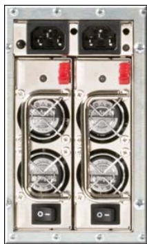
Figure 1. Dual Power Supplies
