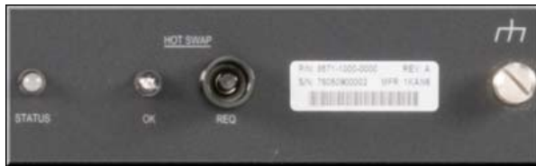
Figure 1. Fan Tray Controls and Indicators
