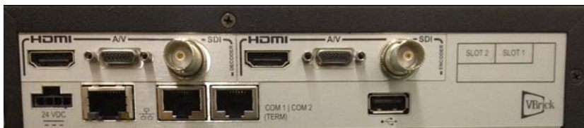
Figure 2. Dual Channel Encoder (with SDI)
