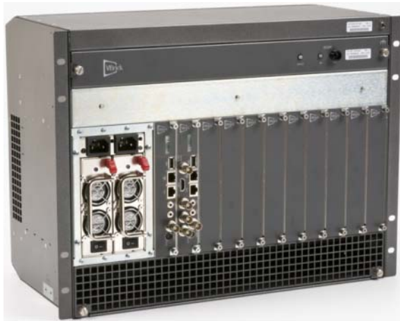
Figure 1. Vbrick 9000 Encoder Rack Mount Shelf
