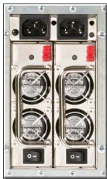
Figure 1. Dual Power Supplies
