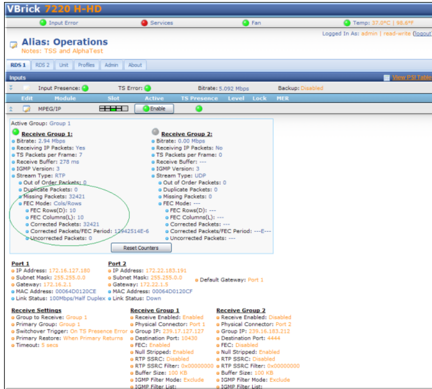
Figure 1. FEC Statistics on Vbrick 7000 Series Decoder
