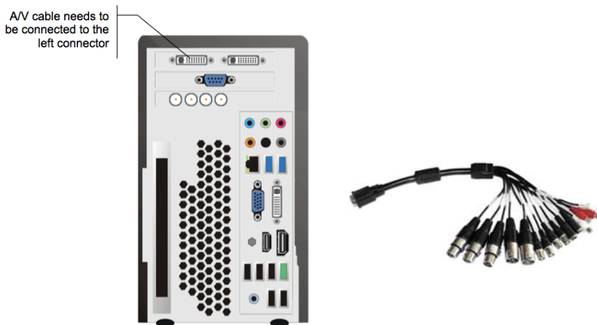
Figure 21. Back Panel with A/V Cable
