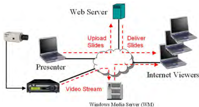
Figure 15. Typical Reflector Configuration
