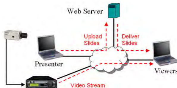
Figure 13. Typical Unicast Configuration
