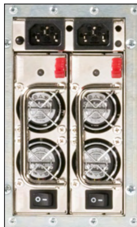
Figure 8. Dual Power Supplies
